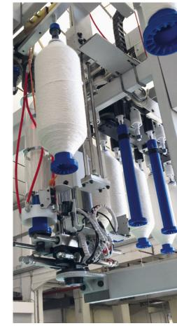
IBC – bobbin stripper integrated on the exchanger
